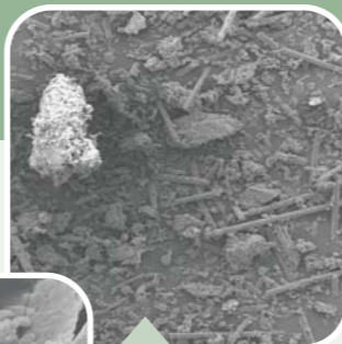
Milled GRP: 100 x magnification. Image shows strand integrity of GRP is retained after milling process
